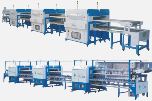
Stockfit / Assembly Cement Drying Unit
